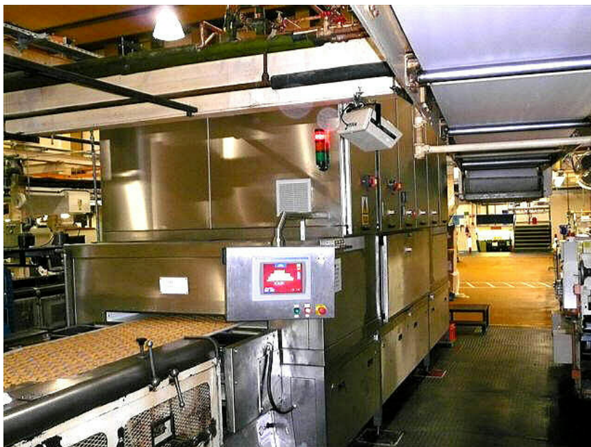
Fig 4. A 50kW RF Dryer (Photo courtesy of Fox's Biscuits and Strayfield Ltd)
