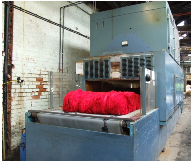
A typical RF Tunnel Oven for Textile Drying (courtesy G3PJD)
