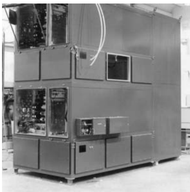
Photo: 100kW Vertical Tube Heater with 300mm dia. tube under construction in the UK
