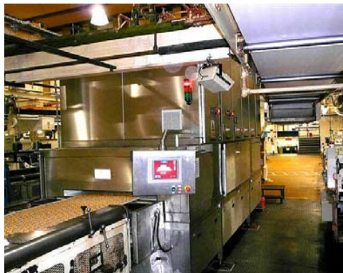
Photo: Latest 50kW RF Post Baking Unit - Courtesy of Fox's Biscuits Batley, Yorkshire, UK
