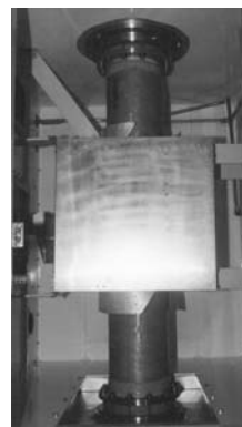
Photo: 100kW Vertical Tube Heater with 300mm dia. tube under construction in the UK
